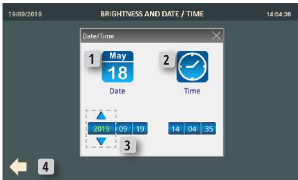
Fig. 52 Date/Time Setting Window
