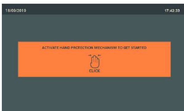
Fig. 31 TFI Hand Protection Guard Check Screen
