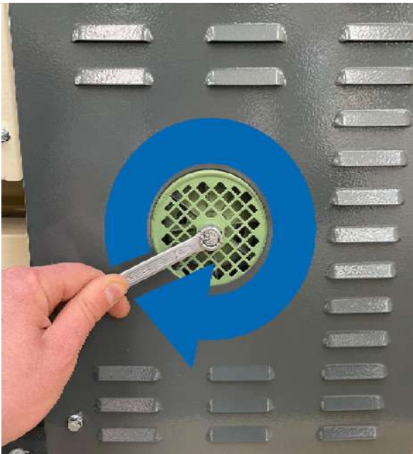
Photo 5 Ring Spanner Usage on the 35xx series
