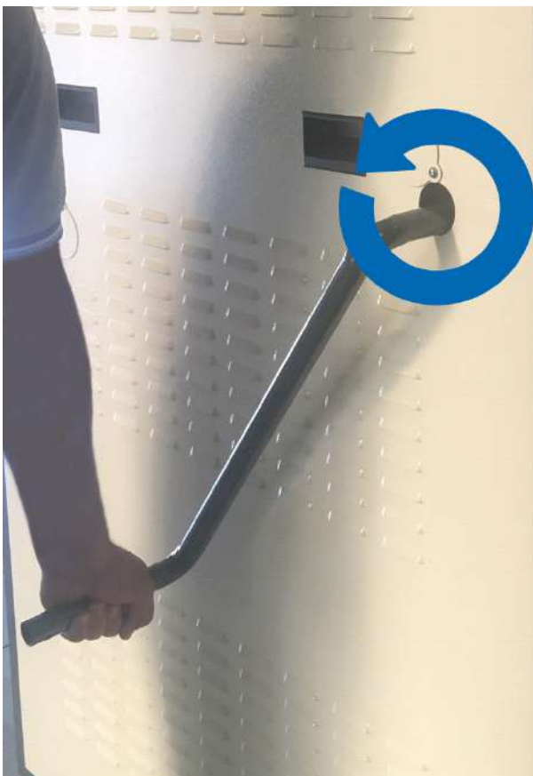
Photo 4 Crank Handle Usage on the 60xx series
