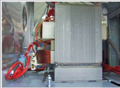
1000W e2s variant: one high voltage transformer feeding the magnetron.
