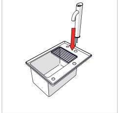
Mount the font on the sink. Placing the threaded bar, hose and wiring through the hole.
