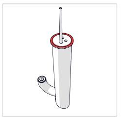
Apply silicone sealant to the bottom of the font in the area marked in red.
